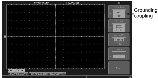
Picture 2-3 channels are being set as grounding
