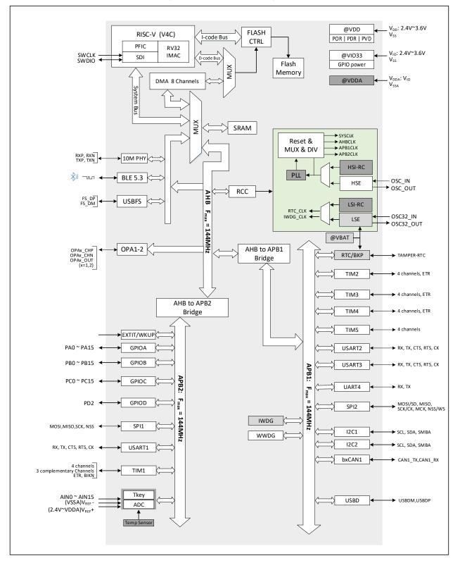
Figure 2-1 System block diagram
