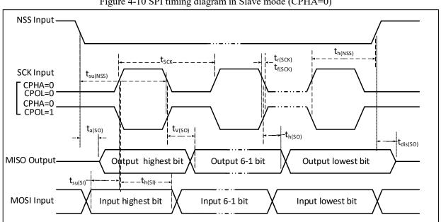
Figure 4-10 SPI timing diagram in Slave mode (CPHA=0)
