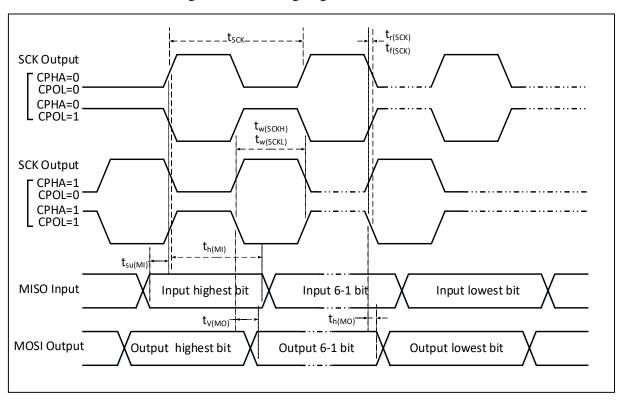
Figure 4-9 SPI timing diagram in Master mode
