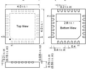
Figure 5-1 QFN28X4 package
