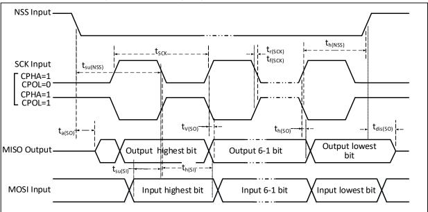
Figure 4-11 SPI timing diagram in Slave mode (CPHA=1)
