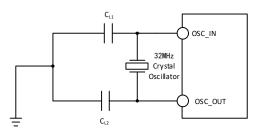
Table 4-12 Low-speed external clock generated by generated from a crystal/ceramic resonator
