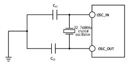
Note: The load capacitance  $C_L$  is calculated by the following formula:  $C_L = C_{L1} \times C_{L2} / (C_{L1} + C_{L2}) + C_{stray}$ .  $C_{stray}$  is the capacitance of the pin and the PCB board or PCB-related capacitance. Its typical value is between 2pF and 7pF.
