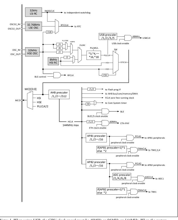
Note: 1. When using USB, the CPU clock speed must be 48MHz or 96MHz or 144MHz. When the system wakes up from Stop mode or Standby mode, the system will automatically select HSI as the system clock frequency. If USB and ETH both are enabled, select USBPRE=5DIV, configure PLLCKR=SYSCLK to be 240M, AHBPRE=2DIV, and the CPU clock speed is 120M.
