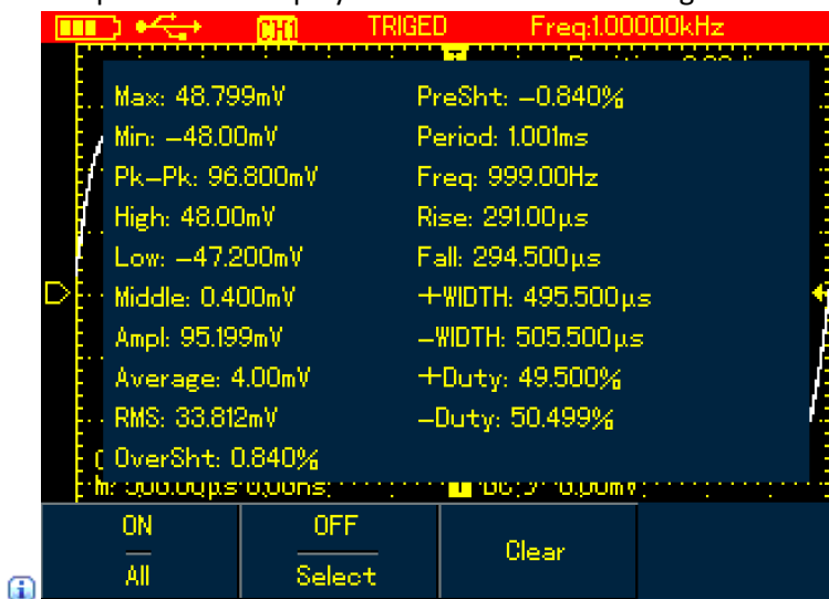
Figure 6-16A UTD1000CL measures all parameters
