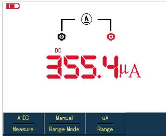
Figure 5-7 Measuring DC Current lower than 4Ma
