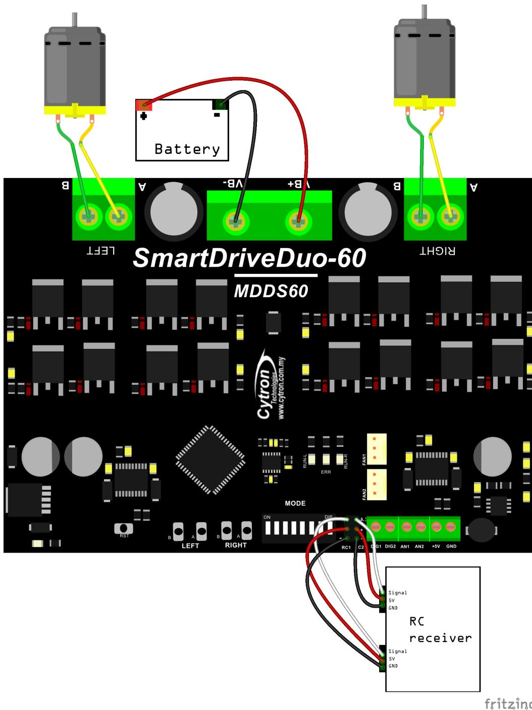
RC Mode with Microcontroller (Independent Both), DIP switch
