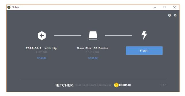
After done flashing, take the SD card out and insert back to your laptop. Open SD card directory (e.g. D:/boot) and open config.txt file. Put enable\_uart=1 at the bottom of the line. Save and eject the SD card. Then insert the SD card into Raspberry Pi Zero WH.
