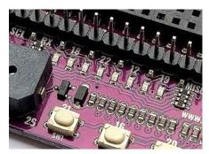
8 LEDs is connected to GPIO 17, 18, 27, 22, 25, 12, 13 and 19. Those LED can be controlled as an output or can be act as an input (signal monitoring). In other words, GPIO that connected to the LED, can be configured as output, input and input pull up.
