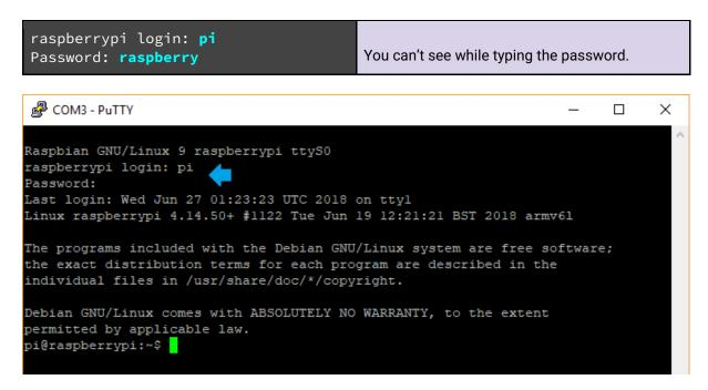
So far, you're able to access Raspberry Pi through serial remote (Maker pHAT). We will further guide you until we can remote using VNC Viewer (Virtual Network Computing).
