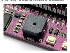
Maker pHAT also comes with on-board active buzzer. It is standard output digital device connected to GPIO 26. To activate it, set GPIO to high, and to mute it, just set GPIO to low.
