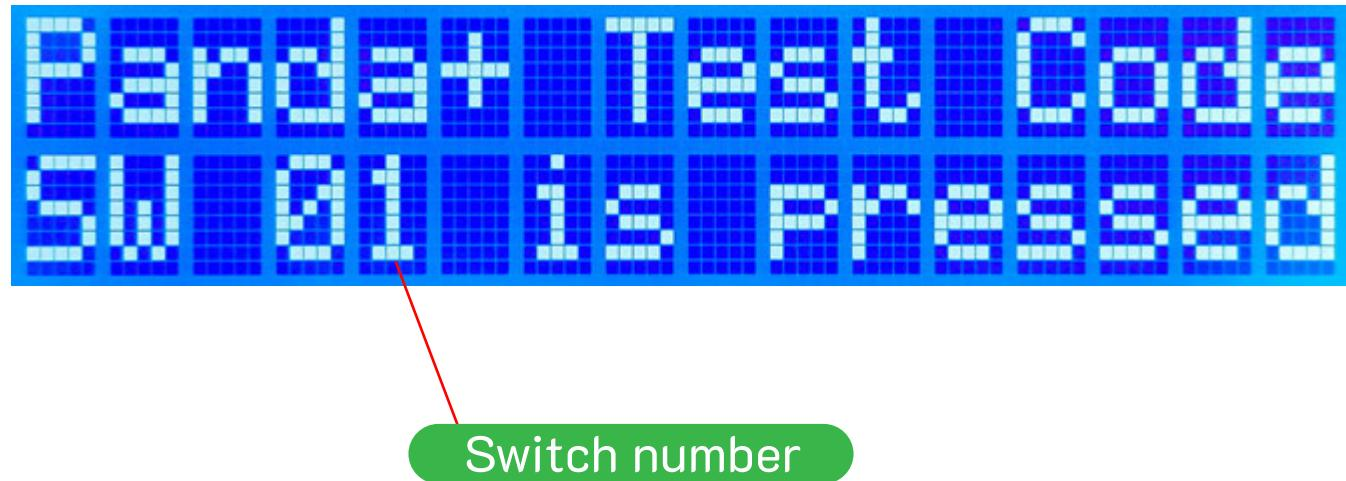
The next table shows the test operation of each switch and LCD message is displayed.
