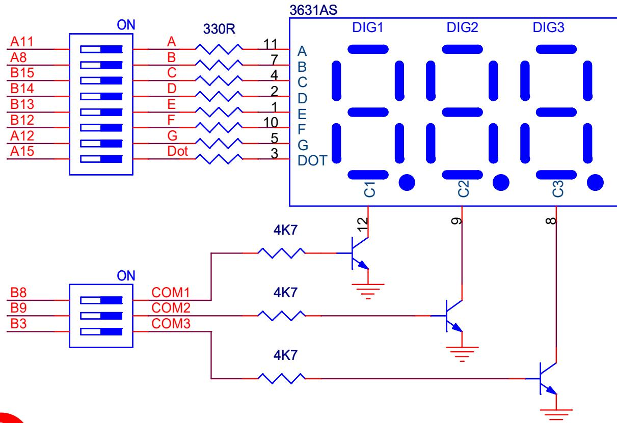
7segment and LCD modules share the same  $\mu$ C port. So, disable LCD before using 7Segment display.
