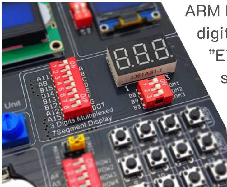
ARM Development Kit provides three multiplexed 7-segment digits. Segments are referred to by letters "A", "B", "C", "D", "E", "F", "G", and "DOT". All digits share the same segment. i.e. segment "A" of DIG1, DIG2, and DIG3 are wired together and driven by the same  $\mu$ C pin. Each digit has its own common cathode which is driven by an NPN transistor. So, a high logic from microcontroller turns transistor on, which in turn enables the digit.
